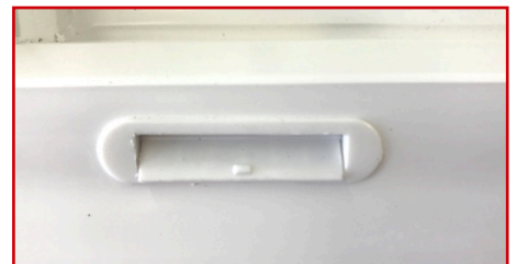
Weep holes are located at the bottom of the sash frame & allow water to escape. We assemble these with a vinyl flap to keep insects and debris out.
